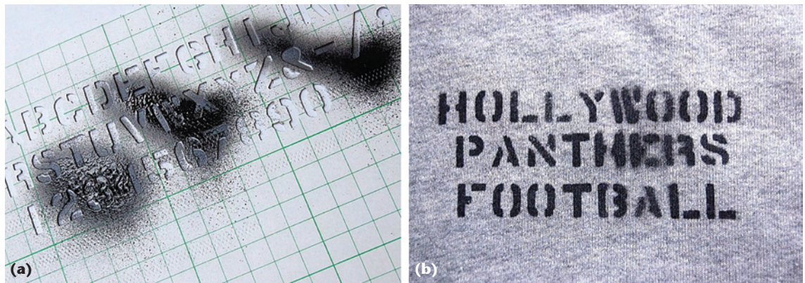
Figure 1. Stencils. (a) In a valid stencil such as this, the template is a single connected piece of material. All islands are connected by a bridge to the main part of the stencil. (b) Using the depicted stencil produces this result. (Source: www.mintclothes.com ; used with permission.)
