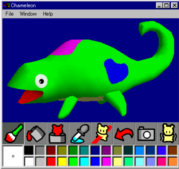
Fig. 2. A screen snapshot of Chameleon. The user paints strokes on the 3D model directly without specifying the UV mapping beforehand.
