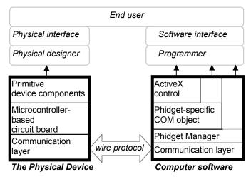
Figure 5. Phidget Architecture
