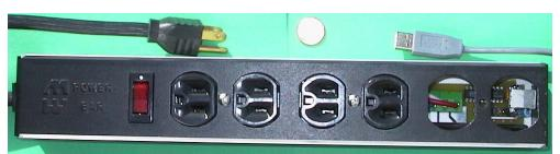
Figure 3: GlabPowerBar. Note the USB connection and the circuit board just visible inside
