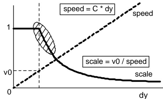
Figure 3: The original mapping from mouse position to speed and scale. A sudden drop in scale (shaded area) occurs when the user first starts moving the mouse.  $dy$  is mouse movement.  $v_0$  and  $C$  are predefined constants.
