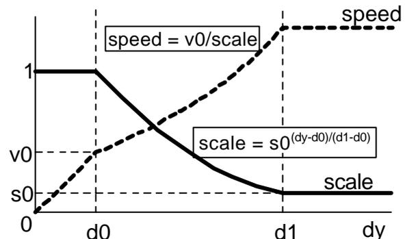
Figure 4: Revised mapping from mouse position to speed and scale. Scale changes at constant rate.  $d_0$ ,  $d_1$ ,  $v_0$ , and  $s_0$  are predefined constants.
