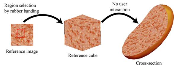
Figure 6 Using an isotropic texture. The user specifies a region to use by rectangular rubber banding, and it is then transferred to all faces of the reference cube and the cross-section.
