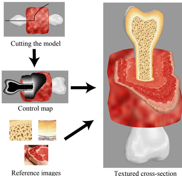
Figure 1 System overview. The user can cut the model anywhere and observe internal textures. Internally, the system first computes a control map using predefined guiding information and then synthesizes the texture using the control map and the reference textures.
