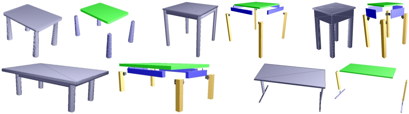
Figure 8: Input 3D models and fabricatable parts/connectors generated by our algorithm for two IKEA table models (MAMMUT, NORDEN) from Google 3D Warehouse and three arbitrary table models (m871, m895, m907) from the Princeton Shape Benchmark. The legs of the MAMMUT table were parsed as cuboids and re-meshed to conic shapes.
