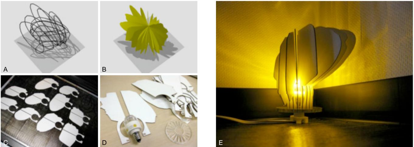
Figure 8. Creating a lamp shade with *Spatial Sketch*, (A) The original 3D sketch (B) Radial slices of the sketch (C) Laser cut slices of card, (D) The final set of parts before assembly, (E) The final assembled lamp shade.
