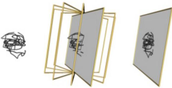
**Figure 5. Slices are created from the original sketch by projecting the sketch on to a series of planes.**
