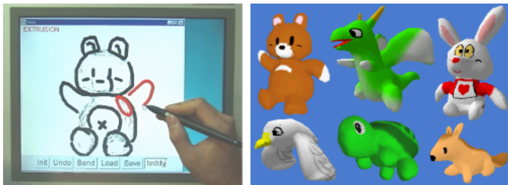
Figure 5: Teddy in use (left) and 3D models created using Teddy (right).
