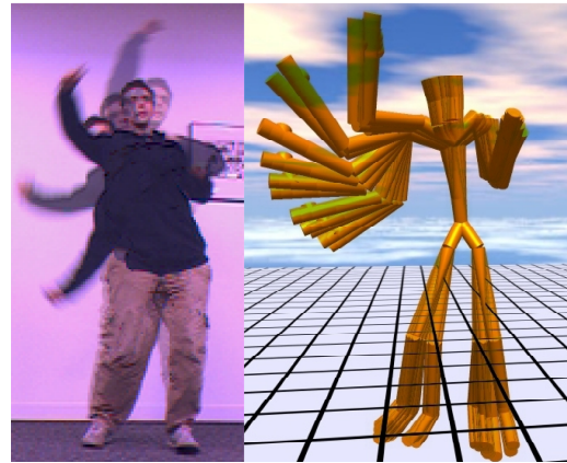
Figure 10: Illustrations of a demonstrated fast moving “punch” movement (left) and the estimated virtual trajectory (right) as traversed by our physically simulated humanoid simulation.
