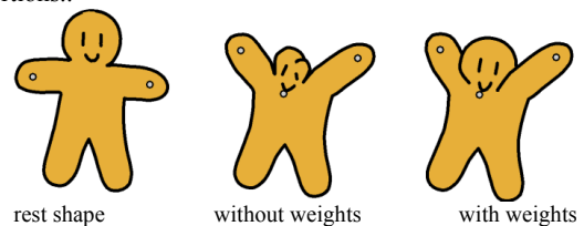
Figure 9: Adjusting rigidity with weights. By adding extra weights to important regions, one can prevent undesirable distortion.
