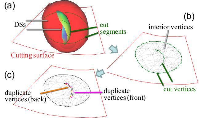
**Figure 3:** Cross-sectional mesh generation. Given DSs and a cutting surface (a), the system triangulates the cutting surface (b) and splits the mesh connectivities (c).
