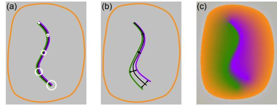
**Figure 2:** A DS is a surface with colors on either side and blur values (a). The blur radii are depicted as white circles. (b) The surface is duplicated into two sheets, which are moved apart along the normals by the blur radius distance. (c) Colors from both sheets are smoothly diffused in space.
