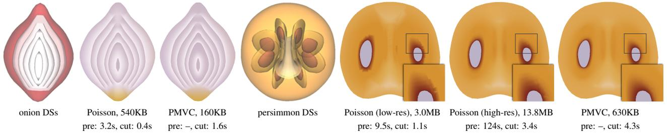
**Figure 4:** Comparisons of our PMVC diffusion and Poisson diffusion. The precomputation time (denoted “pre:”) includes the tetrahedralization and solving the Poisson equation. The storage sizes refer to the precomputed tet mesh with colors for Poisson and the cross-section mesh with colors for our approach.
